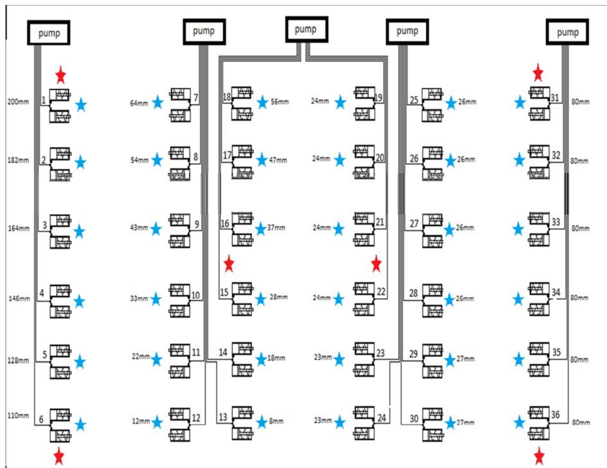
Figure 19: Bridge St Bridge Target Displacement Plan
