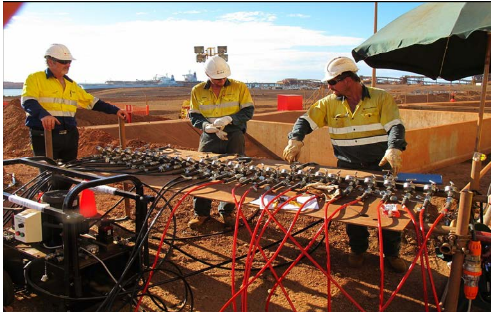
Figure 11: Manual Manifolds with Pressure Gauges off a Split Flow Pump
