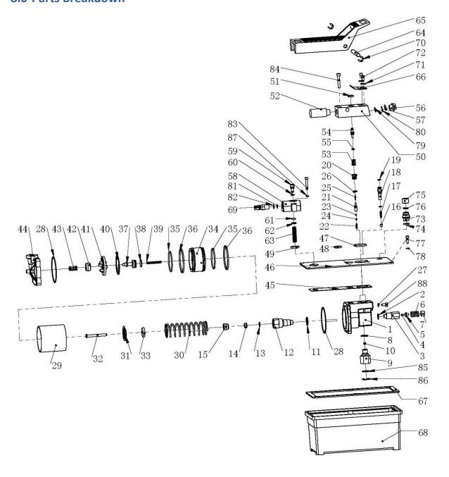
Note: Not all components of the power unit are replacement items but are illustrated as a convenient reference of location and position in the assembly sequence.
