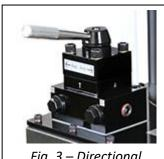
Fig. 3 – Directional Control Valve
