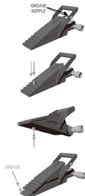
Fig 10-13 – Greasing the Wedge
