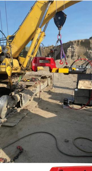
THE **TTP-SERIES** TRACK LINK PIN PUSHER & INSTALLER IS SPECIALLY DESIGNED FOR TRACKED MACHINES, TRACTORS, LOADERS, SHOVELS, EXCAVATORS, ETC. IT IS SUITABLE TO USE WITH MOST MODERN MACHINES INCLUDING JCB, CATERPILLAR, KOMATSU AND POCLAIN MANUFACTURED TRACK MACHINES.
