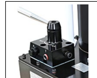
Fig. 3 – Directional Control Valve
